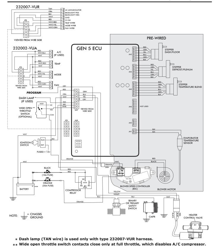
\*\*\* Install fuse assemblies at or as near to the battery as possible.
